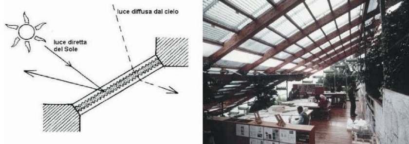
Fig. 16. Working principle and applications of prismatic panels (Renzo Piano workshop Building in Genoa-Italy).
